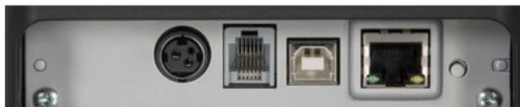
Both models have a USB interface and cash drawer connection. Simply choose between either a RS232 Serial or Ethernet LAN interface.
