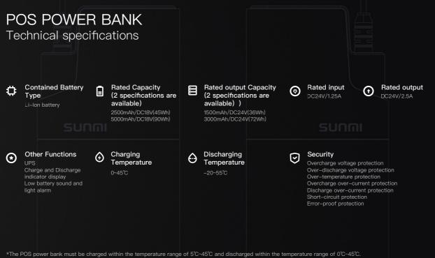
If you charge or discharge the POS power bank beyond this temperature range, it will result in the drastic reduction of battery capacity and the shortening the use time.
